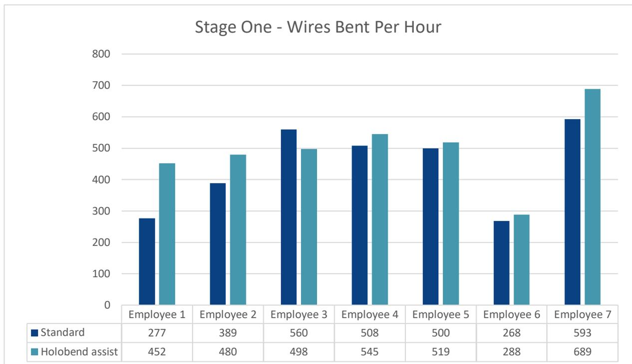
**Figure 3. Comparison of Wires Bent with Headset**
